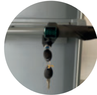
Electronic ignition key and speed adjustment with button for immediate stop
